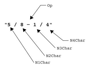
The identifier table shows the variables to be used to store the characters in the string as shown in the diagram.
